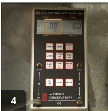
4 Measure CAZ pressure with the door open and record the reading. Close the door and record the reading
