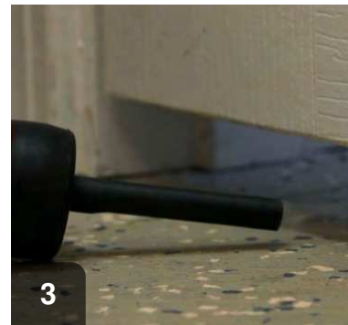
3 Close all doors. With your back to the CAZ, smoke doors with fans behind them. Smoke in:open door, smoke out:close it.
