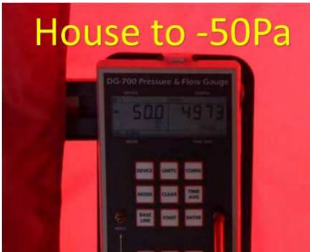
Depressurize the house to 50 pascals.
