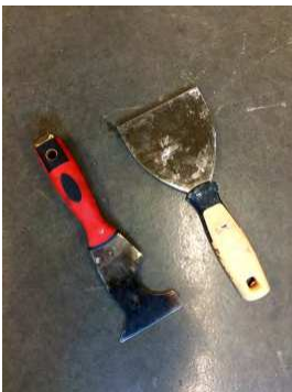
Scrape loose material from insides of cabinet
