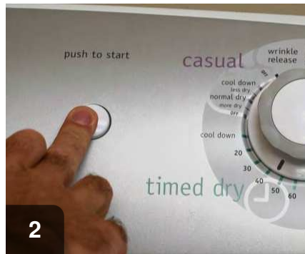
2 Turn on all exhausting appliances(vented outdoors), including the dryer, kitchen fan, and bath fans.
