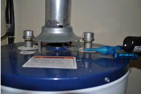
Complete spillage test using chemical smoke pencil
