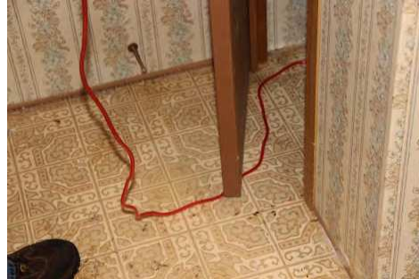
Close the CAZ door or otherwise gain access to the CAZ.
