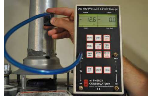
Complete draft test using a manometer
