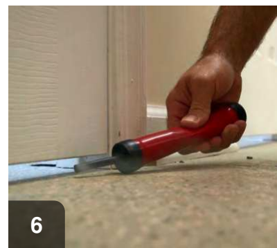
6 Recheck all door positions for worst case depressurization. Smoke hits your toes, leave the door closed.
