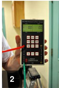
2 Attach test hose to be used in the interior of the house
